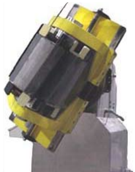
ASSEMBLY MOUNTED ON WINDING MACHINE
